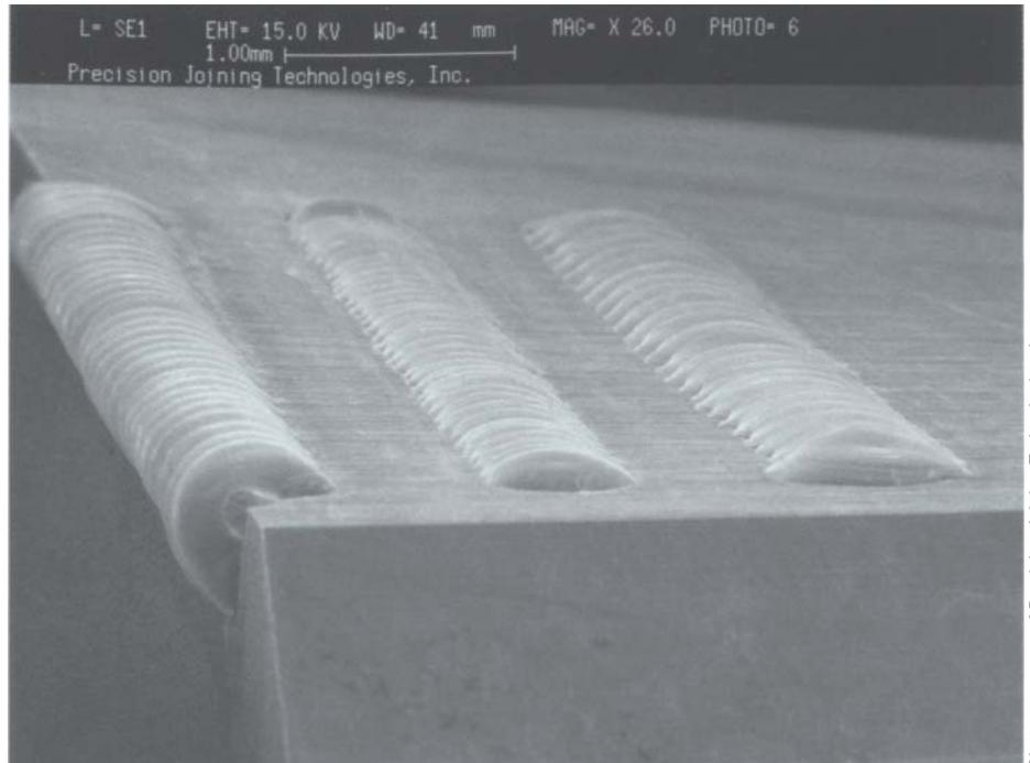
Figure 1 Photograph of typical laser weld build-up of 420 SS mold.
