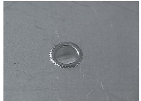
Figure 6 Laser weld repair of the inside diameter of an 1/8-in. hole.
