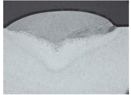
Figure 4 Metallographic cross-section of 0.015-in. filler wire weld shown in Figure 1.
