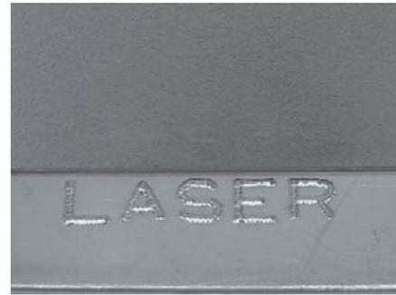
Figure 5 Laser weld repair of an engraving.
