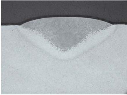
Figure 3 Metallographic cross-section of 0.010-in. filler wire weld shown in Figure 1.
